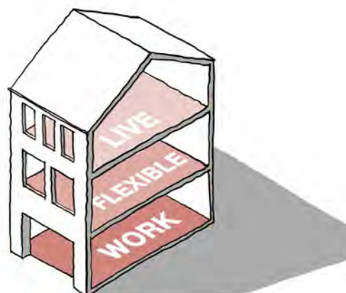
▲ Live / Work typologies, or houses designed with increased ground floor ceiling heights allowing for later adaptation provide a resilient form of accommodation adaptable to changing circumstances and give opportunity to create more vibrant streets and communities.
